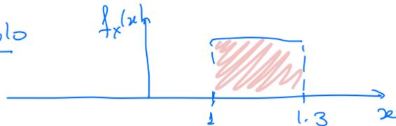
$$\begin{aligned} \text{difer.} &= (1.3 - 1) \cdot k = 0.3 \cdot k = 1 \Rightarrow \\ k &= \frac{1}{0.3} = 3.33 \dots \end{aligned}$$
